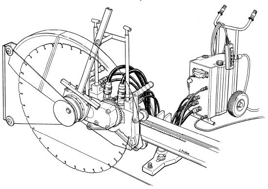
Warning! The power pack must not be connected to the electrical supply until all hoses are first connected to the saw and power pack.
