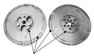
Two friction surfaces: Tighten with torque wrench to 60-70 Nm Must be kept clean!
