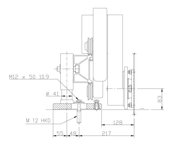
**Warning!** If HKD anchors or another high quality expansion anchor can not be fixed securely, the track feet must be securely fixed with through bolts and large washers to achieve the required level of safety.
