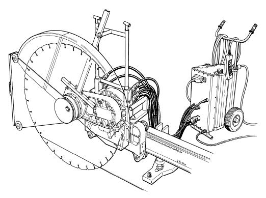
**Hydraulic connections:** Hydraulic power to the blade motor is supplied by two identical <sup>3</sup>/<sub>4</sub>" 8 m long hoses. The feed and travel motors are supplied by 2 + 2 3/8" hoses with the same length, packaged together with a 10 mm water hose. All hydraulic couplings are arranged in such a way that they can only be connected in the correct way.
