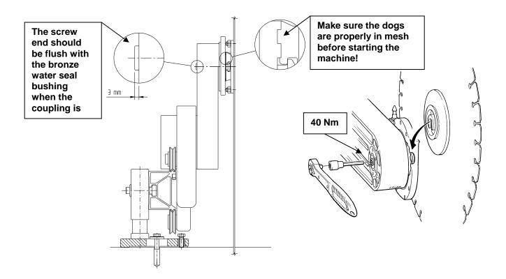
*Warning!* Never fit the blade and flange to the saw spindle before first disconnecting the two 3/4" hoses (the two biggest) from the saw. This important rule must always be strictly followed to ensure that the blade motor cannot be inadvertently started. Failure to follow this instruction may result in serious personal injury or death.
