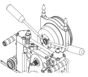
4. If the wear sleeve needs to be replaced, the wear sleeve can be pulled off using a special tool, Part No. 65420100. The new wear sleeve should be installed flush with the clamp screw as shown in the picture below.
