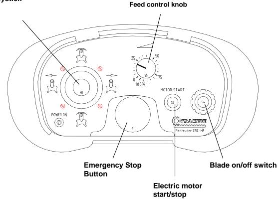
**Start of blade:** To start the blade motor, press the Blade on/off switch button and keep it pressed, then press the Electric motor start/stop button once again.
